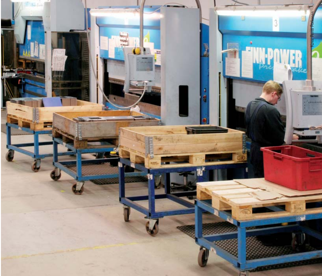
In the major layout change at the Heinävesi factory, such equipment as press brakes were collected in one area.
